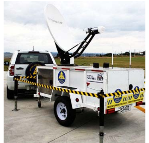
This 1.2 meter T-100 is often used for mobile command posts in regions hit with disasters. The T-100 provides both broadband Internet and VoIP phone service.
