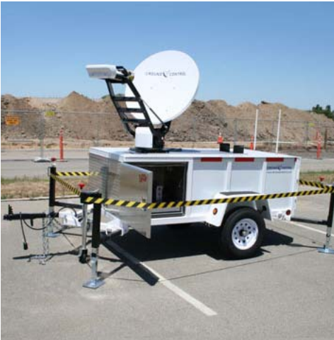
The T-100 is fully self-contained and easy to operate. One-Button deployment and a half-mile radius 802.11 wireless connectivity requires no special certification or licensing to use.
